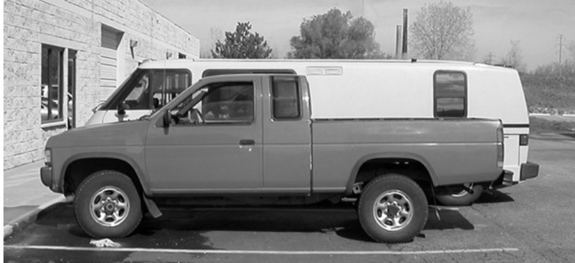
This truck has a higher drag than the streamlined RV behind it.
